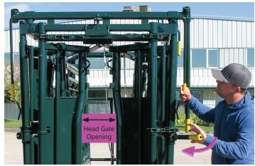
2 > Push the head gate operation handle forward and towards the chute. Rotate the head gate into the chute until the opening width matches your self-catch requirements.
