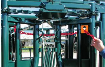
4 > With the limiter chain tight, and the head gate opening set to the self-catch width, lock the limiter chain in the keyhole latch.
