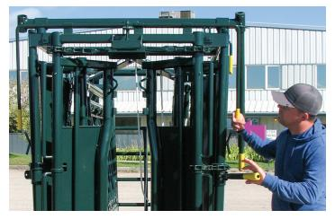
1 > Release the head gate by pushing the head gate release handle towards the back of the chute. While holding the head gate in the released position perform step 2.
