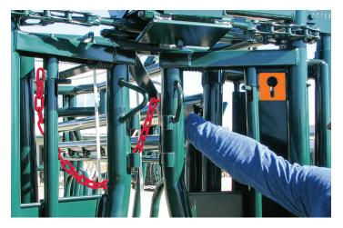
3 > Pull the limiter chain across the chute on the INSIDE of the head gate.
